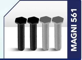
Magni 561 is a duplex coating that combines electroplated tin/zinc and hex-chrome-free passivated substrate with an organic topcoat. It can be engineered to specific coefficient-of-friction needs. Magni 561 is engineered for use on parts that interact with magnesium. Magni 561 is typically applied to fasteners, including nuts, bolts and other hardware. Magni 561 can be applied via dip-spin or spray application methods.
